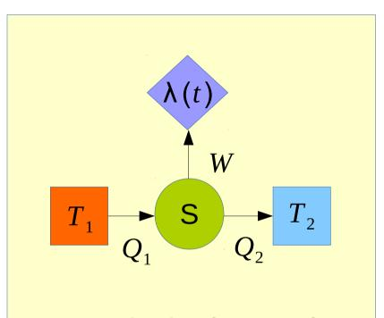
System is simultaneously in contact with multiple heat baths.
