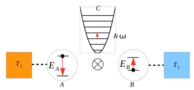
$$\frac{\partial}{\partial t}\rho_S(t) = -\frac{i}{\hbar}[\mathcal{H}_S, \rho_S] + \mathcal{D}_{T_1}^{\mathcal{H}_A}[\rho_S] + \mathcal{D}_{T_2}^{\mathcal{H}_B}[\rho_S]$$
